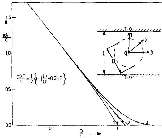
FIG. 2. Steady-state temperature for three positions at a distance  $D/2$  from a continuous line source with strength  $1/(\rho C_p)$ , the source being positioned in the middle between two plates at zero relative temperature.
